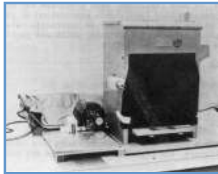
Figure 15. Waco Saw for sectioning, to left, and seam projector for examining cross sections of double seams, to right in photograph.
